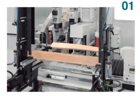
Standard machine: Frontal hopper feed loader, horizontal router head, vertical (tilt) router head, shaping head, turning and flat sanding unit. Optional: Sanding unit for turned parts
