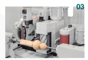
Detail of machining a turned table leg using the turnery saw blade and sanded by the narrow sanding belt unit.
