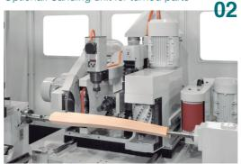
Detail of machining a table leg using the shaping head and sanded by the flat sanding unit.
