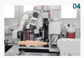
Detail of machining a table leg with the tilted vertical router head.
